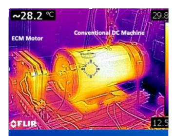
In this picture, both machines are processing 500W. You can see that in the conventional machine (right) the heat is mostly internal. In the ECM machine (left) most of the heat is at the outer radius of the machine.
