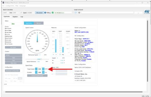
9. Click "Start Motor" to start the motor. Motor will accelerate to the speed set in step 8.
