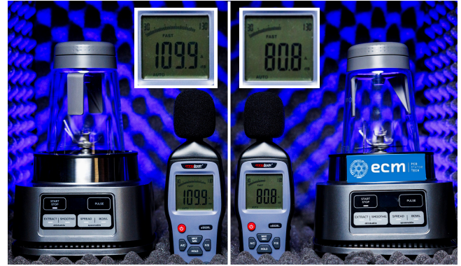
In a recent test, the blender unit powered by ECM's PCB Stator motor operated 29 dB quieter than a conventional motor.
