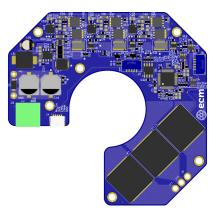
The shelfstock servomotor is capable of either 0-10V speed control or CANopen-based control. The following guide is intended for a motor configured for CANopen-based control. To operate this motor, you will need a 36V motor power supply and a CANopen capable interface to control the motor.
