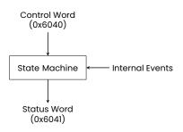
The state machine describes the state evolution of the device with respect to the control of power electronics due to user commands and internal drive faults.
