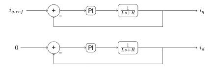
The stator's electrical transfer function, i(s)/v(s) = 1/(Ls + R), where L and R are the phase-to-neutral inductance and resistance, respectively, includes the extra series inductance present on the drive. The PI controller gains are, by default, chosen to cancel the poles in the stator's transfer function, or
