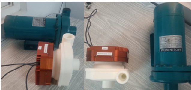
Compact PCB Stator motor integration next to legacy pump motor
