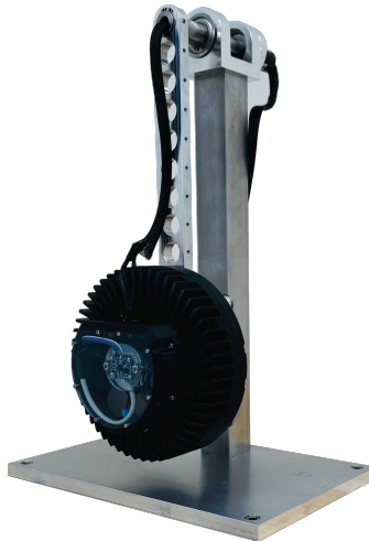
Figure 1: ECM's reaction wheel inverted pendulum.
