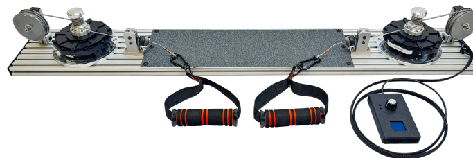
Figure 3: ECM's prototype cable-driven weightlifting machine integration. Weights are simulated via ECM 2 Nm (nominal) shelf stock motors.
